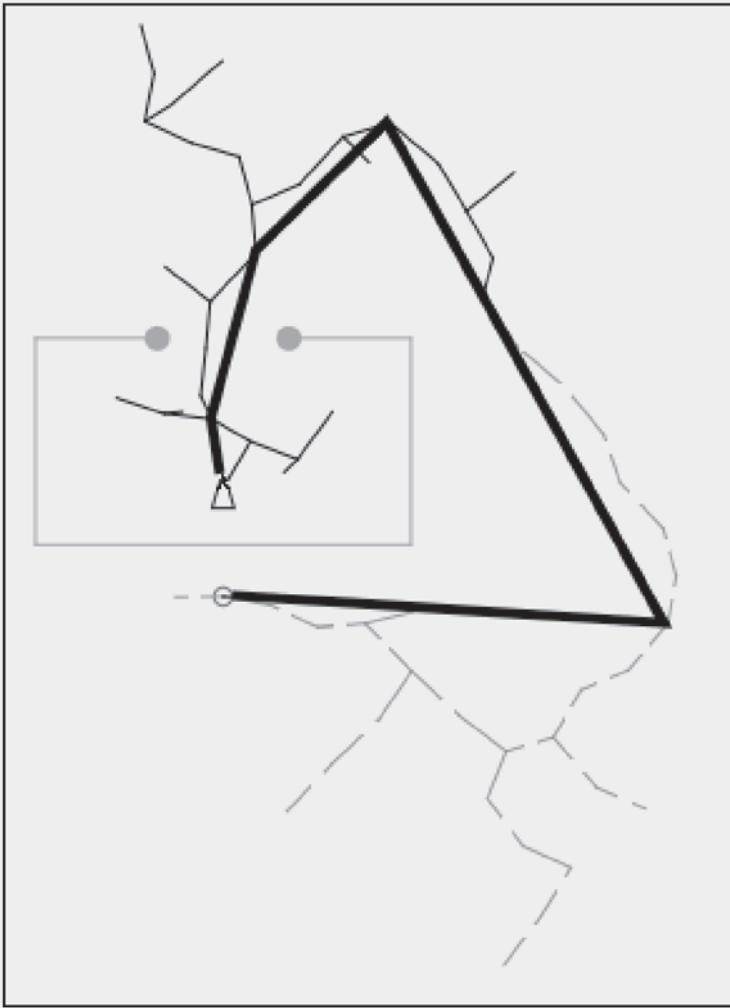
Figure 1. Using the RRT-Connect algorithm to escape from a box. The robot's current pose is shown by the small triangle, and a goal location below the box is shown as a hollow circle. The search tree rooted at the robot's location is shown as a thin black line, while the search tree rooted at the goal is shown as a dashed gray line. When the trees meet, a solution has been found. After applying a smoothing algorithm, the resulting solution path is shown as a thick line.
