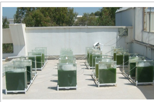
Figure 10—Flat-plate photobioreactor. Photo taken at the Microalgal Biotechnology Lab of the Faculty of Fisheries of Çukurova University in Adana, Turkey.
