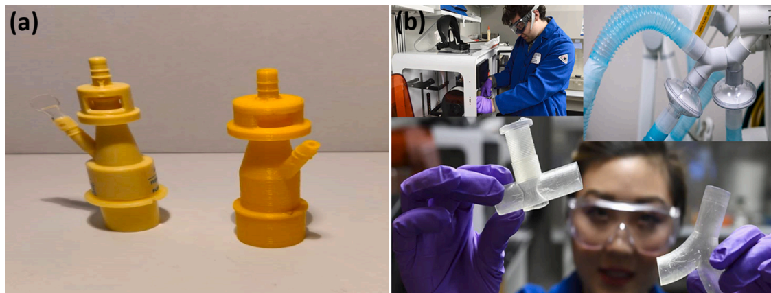
Fig. 5. COVID-19, a respiratory-related disease, creates enormous demands for ventilators. Ventilators and their various components are some of the most essential and life-saving medical equipment. (a) An additively manufactured ventilator valve perfectly replicates an original valve made by traditional manufacturing techniques, (b) 3D printing technology efficiently creates ample options by manufacturing T-connector, Y-connector, etc. for using a single ventilator for multiple patients (Photo credit: Isinnova, VESper).
