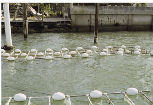
Fig. 2. (Left): Change in percent original tensile extensibility of polypropylene tape exposed in air and floating in sea water in Biscayne Bay, FL. (Right): The floating rig used to expose plastics to surface water environment (Miami Beach, FL).
