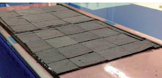
Figure 4: An example of a discontinuous coupon layout, pre-infusion, made up of 100mm square triaxial NCF patches (nearest) and 150mm square triaxial NCF patches (furthest).
