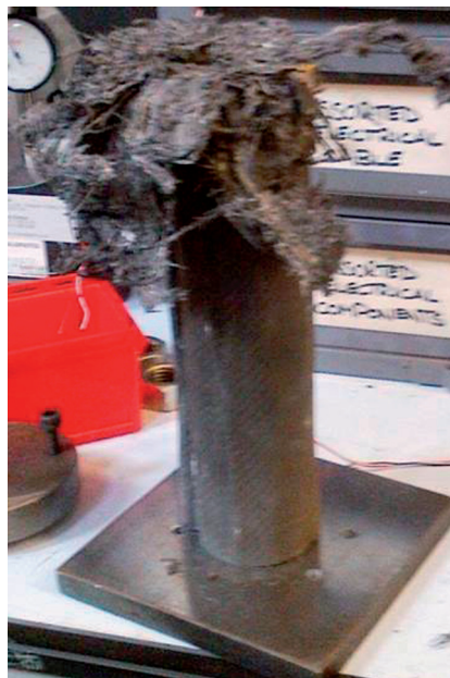
Figure 6: Image of a demonstrator crush tube, after quasi-static testing at 18mm per second.
