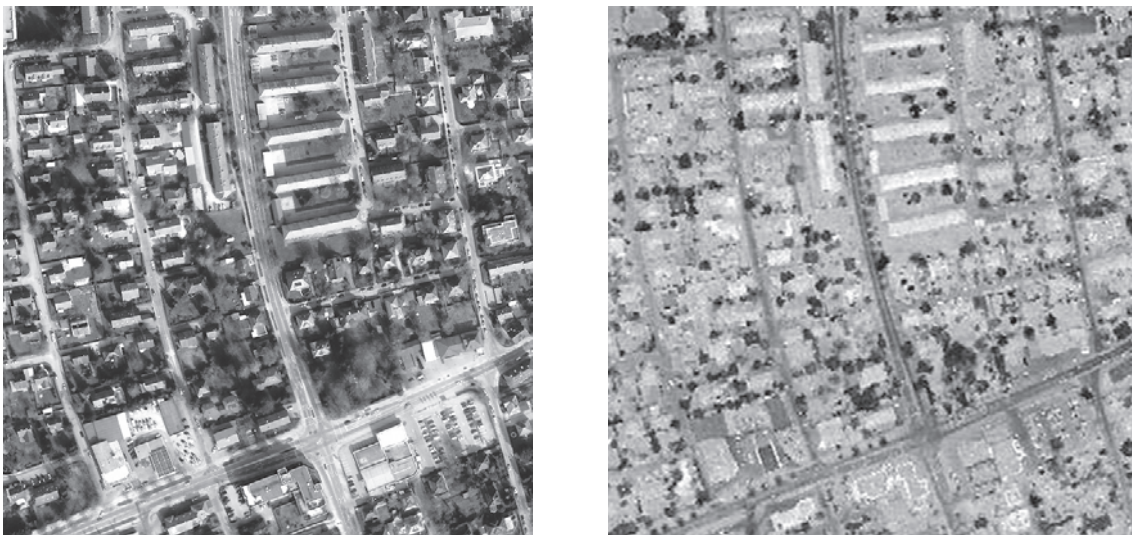
Figure 1.6 Aerial image (left) and LIDAR intensity image (right) of a built-up area. Source: TopoSys.
