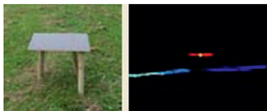
Figure 4.3 Ground control and checking in corridor projects using ALS. Targets with elevation difference to the ground and special reflecting material (left) can precisely be identified in the dense point cloud (right). Source: Flatman 2009
