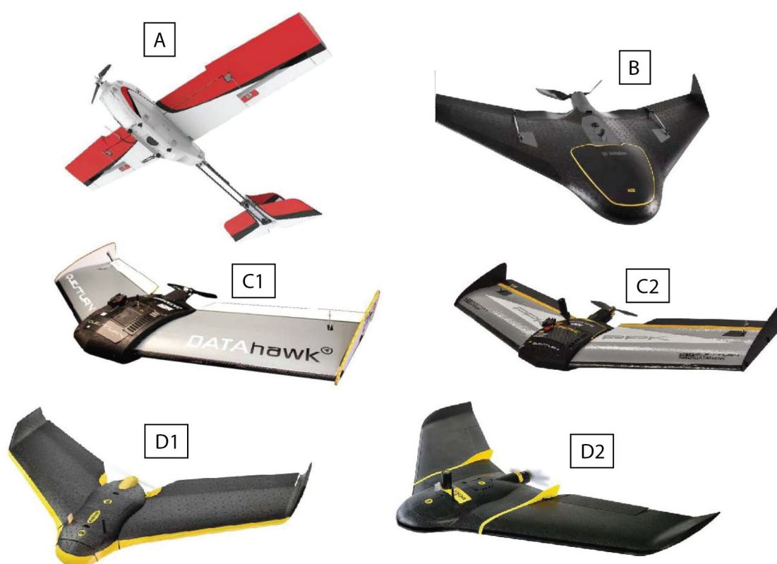
Figure 4. Examples of fixed wing UAS: (A) Precision Hawk Lancaster 5; (B) Trimble UX5; (C1) QuestUAV DATAhawk; (C2) QuestUAV DATAhawk PPK; (D1) senseFly eBee; (D2) senseFly eBee Plus.
