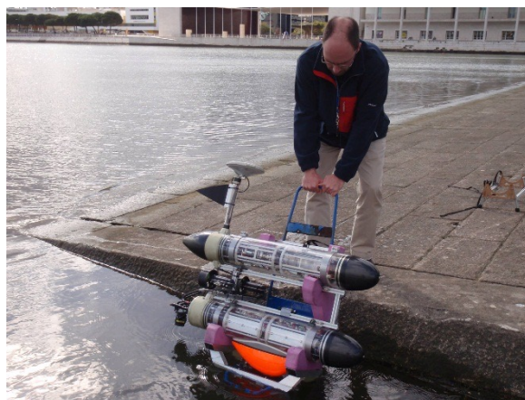
The same cart can be used to deploy/recover the vehicle
