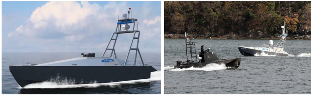
Figure 14: The Aragon USV (left); Automatic Collision Avoidance Test (right). Photo courtesy of Jinwhan Kim, KAIST.
