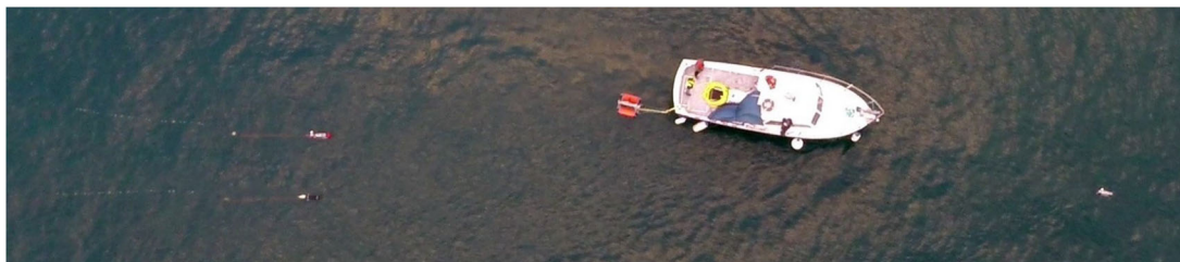
FIGURE 13 A manned boat towing a sparker in coordination with the autonomous underwater vehicles (AUVs) during the first full-scale integration campaign. These tests were instrumental to the decision of substituting the manned boat with autonomous surface vehicles due to the difficulty in coordinating manned vehicles with the AUVs
