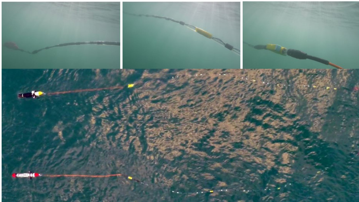
FIGURE 14 Images of 16 m long streamers towed by the autonomous underwater vehicles (AUVs) during the first integration campaign: aerial (bottom) and underwater (top) views. As in images shown, the streamer shape while being towed was far from ideal due to the low speed of the AUVs. After these trials, it was decided to reduce the streamer length to 8 m
