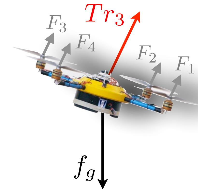
$$\begin{aligned} r_3 &= Re_3 = R \begin{bmatrix} 0 \\ 0 \\ 1 \end{bmatrix} \\ f_g &= mge_3 \end{aligned}$$
